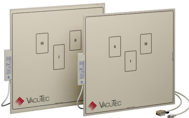
The AEC chambers are air-filled parallel-plate ionization chambers with typically one or three independent sensor fields. Several different outer dimensions are available. Each VacuTec AEC chamber is equipped with a preamplifier and electronics, which converts the low ionization current into EMC stable digital signals. Additionally it supplies the voltage for the chamber operation and allows selection of the sensor fields.
